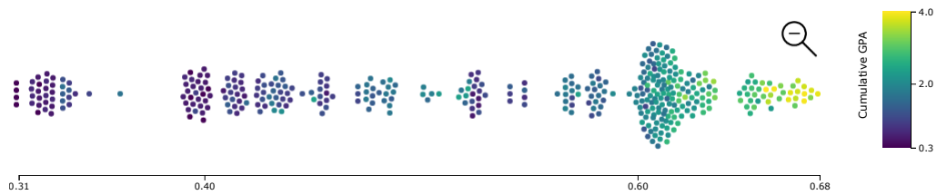
FIGURE 5.1: An example of a beeswarm plot. Points are spread out along a horizontal axis, clustering in swarms when multiple points have the same value.
