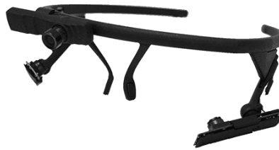
Figure 2: Pupil Core provides eye-tracking data that can estimate gaze/fixation points over the network. It also captures images from the world at thirty frames per second at 720p.
